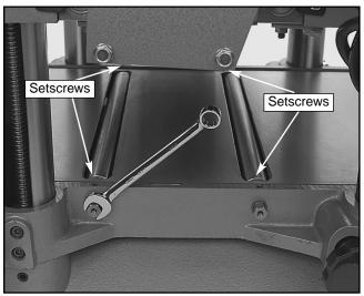
Figure 28. Adjusting bed roller height.
